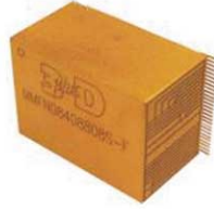
Figure 12: Radiation tolerant NAND chip [17].
